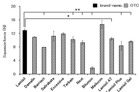
**Figure 5. Squeeze force for various creams (n = 3).** \* $p < 0.05$ , \*\* $p < 0.01$  (vs. Lamisil cream, Dunnett's test).
