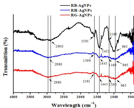
Figure 4. FTIR of the obtained AgNPs.
