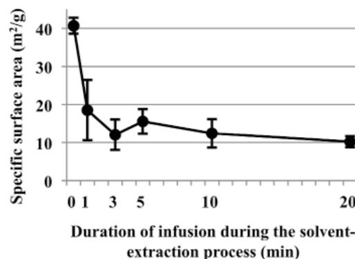
**Figure 4. Effects of the infusion period during the solvent-extraction process on the specific surface area of the microspheres.** The point at time 0 indicates the specific surface area of the EC microspheres prepared in mode 1. The points at other times indicate the specific surface areas of the EC microspheres prepared in mode 2. The data shown represent the mean  $\pm$  SD ( $n = 3$  batches).
