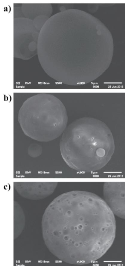
**Figure 2. Scanning electron micrographs of the fabricated EC microspheres.** The EC microspheres shown were prepared by (a) the proposed method (mode 1), (b) the conventional O/W-type emulsion solvent evaporation method, and (c) the conventional W/O/W-type emulsion solvent evaporation method. The bars represent 5  $\mu\text{m}$ .
