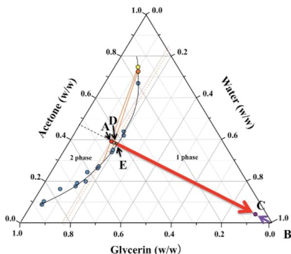
**Figure 5. Triangular diagram of the acetone-glycerin-water ternary system.** The data corresponding to the border line between phases 1 and 2 were taken from the literature (12). The concentrations of acetone, glycerin, and water for the various points were as follows: point A (acetone/glycerin/water = 0.399:0.424:0.178), point D (acetone/glycerin/water = 0.388:0.424:0.188), and point E (acetone/glycerin/water = 0.386:0.422:0.193).
