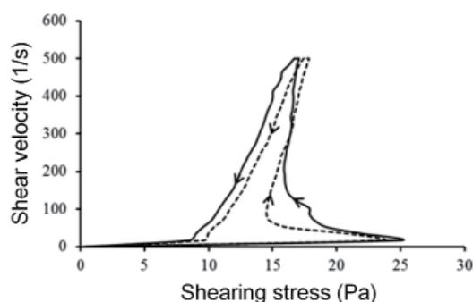
**Figure 1. Thixotropic change of lithium magnesium sodium silicate gels prepared using electrolytic-reduction ion water (GE-100) sonicated by ultrasonication.** Dotted line: before ultrasonication; solid line: after ultrasonication. Each linear arrow showed a direction of the hysteresis loop.
