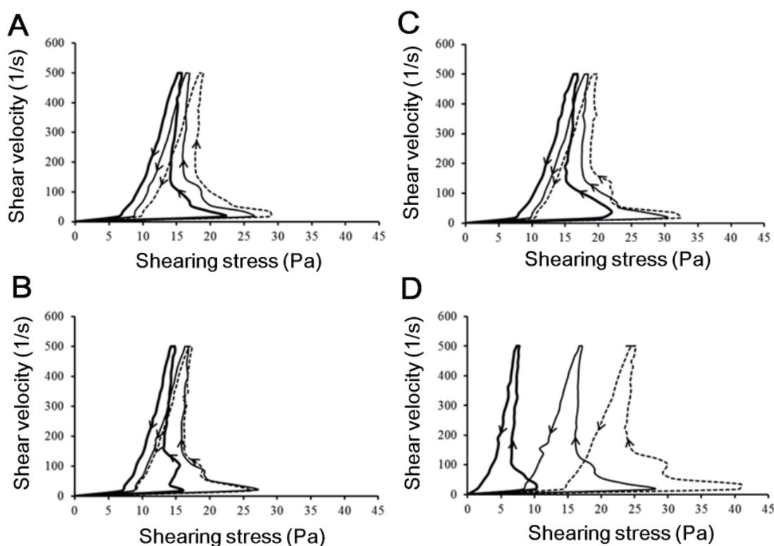
**Figure 2. Thixotropic changes of different gels containing various oils.** Dotted line: GE-100 + 0.1% oil; thin solid line: GE-100 + 1% oil; thick solid line: GE-100 + 10% oil. (A): jojoba oil, (B): squalane, (C): olive oil, (D): MCT. Each linear arrow showed a direction of the hysteresis loop.
