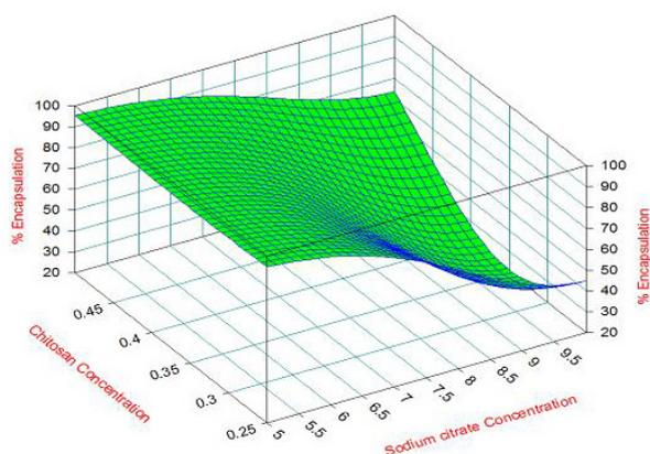
**Figure 3.** Effect of the interaction between sodium citrate concentration and chitosan concentration on %encapsulation efficiency of DFS-C microspheres.
