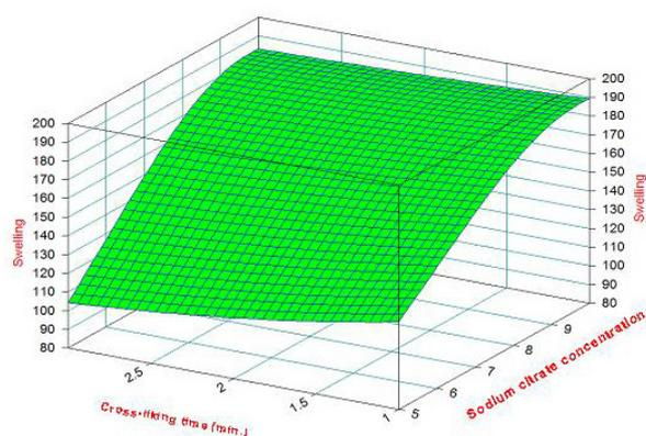
**Figure 4.** Effect of the interaction between sodium citrate concentration and cross-linking time on %degree of swelling of DFS-C microspheres.
