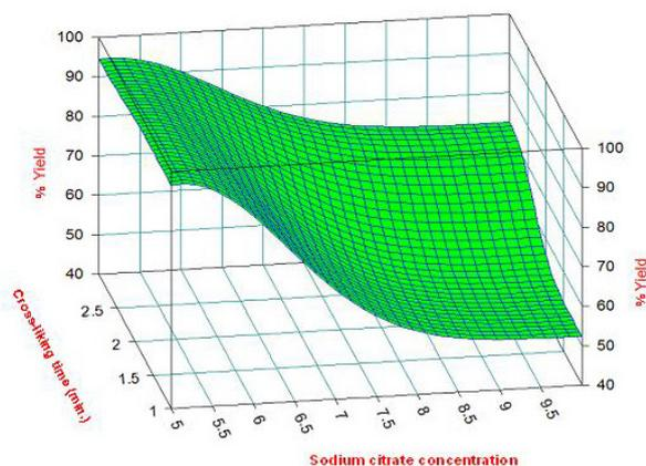
**Figure 2.** Effect of the interaction between sodium citrate concentration and cross-linking time on %yield of DFS-C microspheres.
