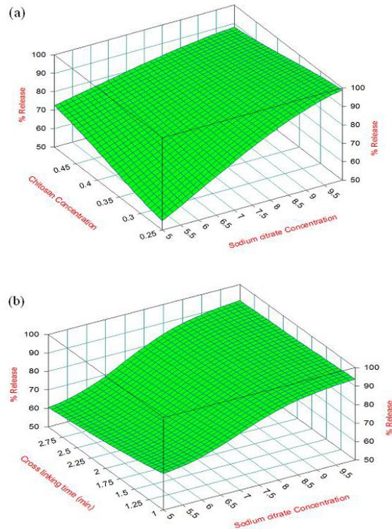
**Figure 6.** Effect of the interaction of sodium citrate concentration with (a) chitosan concentration and (b) cross-linking time on the percent of drug released after 6 h.
