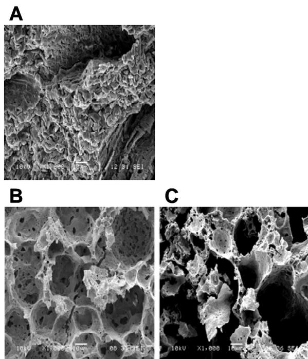
**Figure 3. Effect of manufacturing technique on surface porosity of 5-FU loaded implants. (A)** SEM picture of a PLA implant prepared by injection molding (F1). **(B)** SEM picture of a PLA implant prepared by injection molding (F2). **(C)** SEM picture of a PLA implant prepared by compression (F8).
