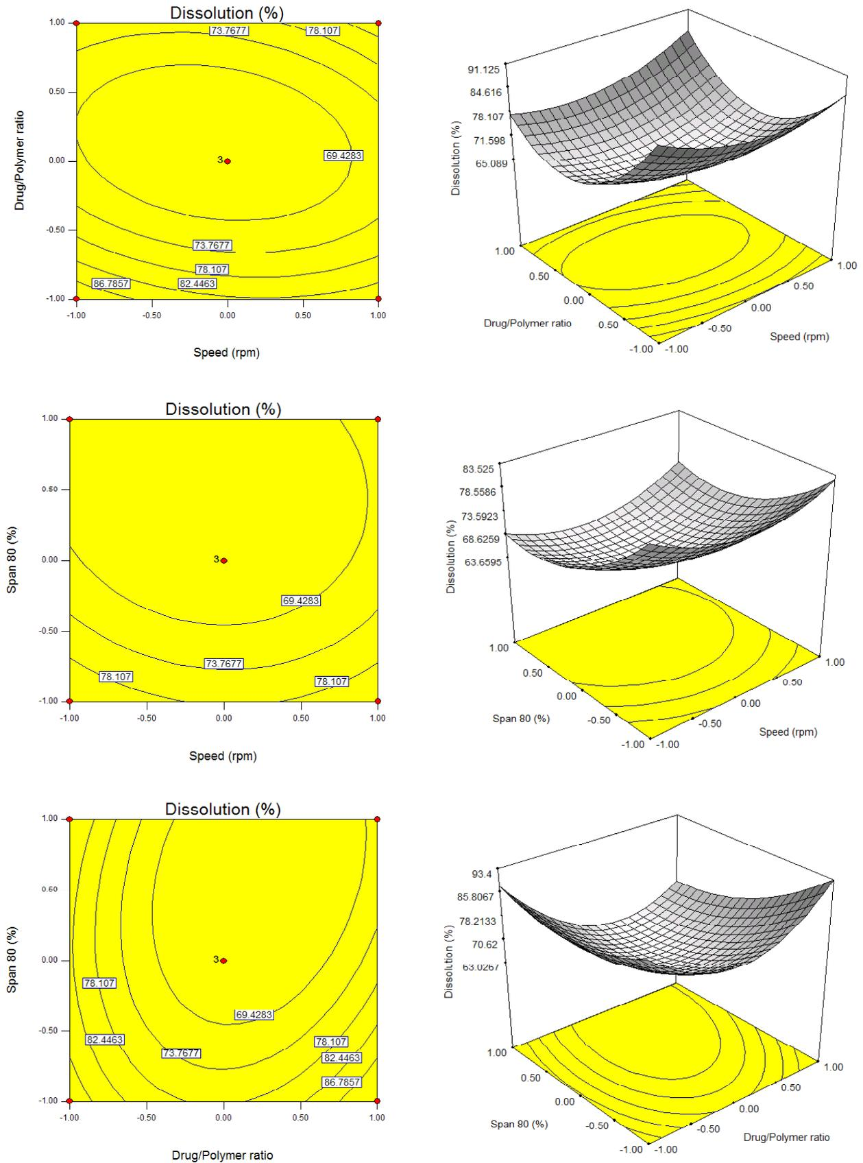
Figure 6. Response surface plots showing the effect of different levels of independent variable (X) on percent drug release from TS microspheres after 8 h (Y<sub>2</sub>). X<sub>1</sub> = speed (rpm); X<sub>2</sub> = drug: polymer; X<sub>3</sub> = % span 80.
