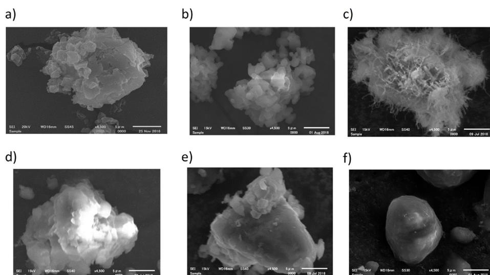
**Figure 1. Scanning electron micrographs of the pulverized quinine and the coated particles. a)** 2 h-pulverized quinine particles, **b)** 8 h-pulverized quinine particles, and the quinine and carnauba wax (1:1) coated particles prepared at 250 rpm for **c)** 0.5 h, **d)** 3 h, **e)** 6 h, and **f)** 12 h. Morphology changed during the dry coating process was demonstrated.
