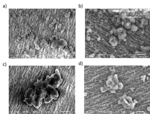
**Figure 3. Scanning electron micrographs of the coated particles.** The particles prepared by a) standard conditions, b) process time of 12h, c) milling speed of 500rpm, d) quinine-to-carnauba wax ratio of 1:4. The conditions of 1:1, 250 rpm, and 6 h for quinine/carnauba wax ratio, milling speed, and process time, respectively, were selected as the standard.
