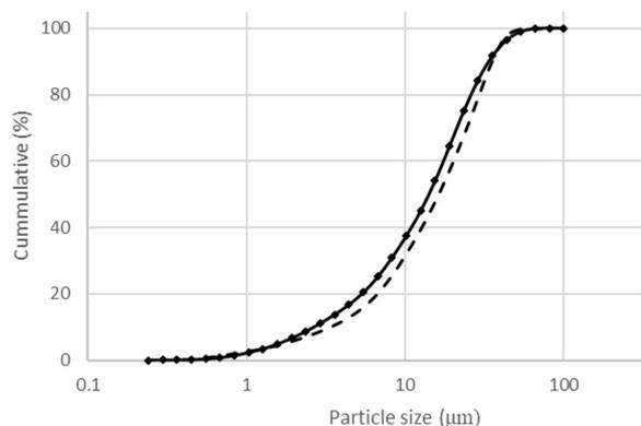
**Figure 4. Cumulative particle size distribution of the typical coated particles.** The solid and dot lines express the actual size and theoretical size distribution, respectively. The coated particles were prepared by the condition: quinine/carnauba wax ratio 1:1, milling speed 250 rpm, process time 12 h.
