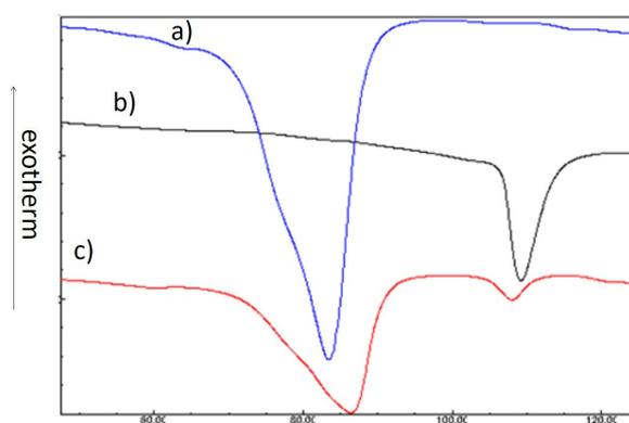
**Figure 6. DSC charts.** a) carnauba wax, b) quinine, c) the coated particles prepared by the standard condition: quinine/carnauba wax ratio 1:1, milling speed 250 rpm, process time 6 h.
