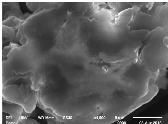
**Figure 2. Scanning electron micrograph of the cross section of the coated particles.** The coated particle of the quinine and carnauba wax (1:1) were prepared at 250 rpm for 12 h.
