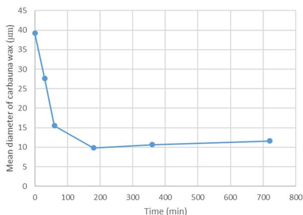
**Figure 5. Change in size of carnauba wax particles during the dry coating process.** Quinine-to-carnauba wax ratio and milling speed were 1:1 and 250 rpm, respectively.
