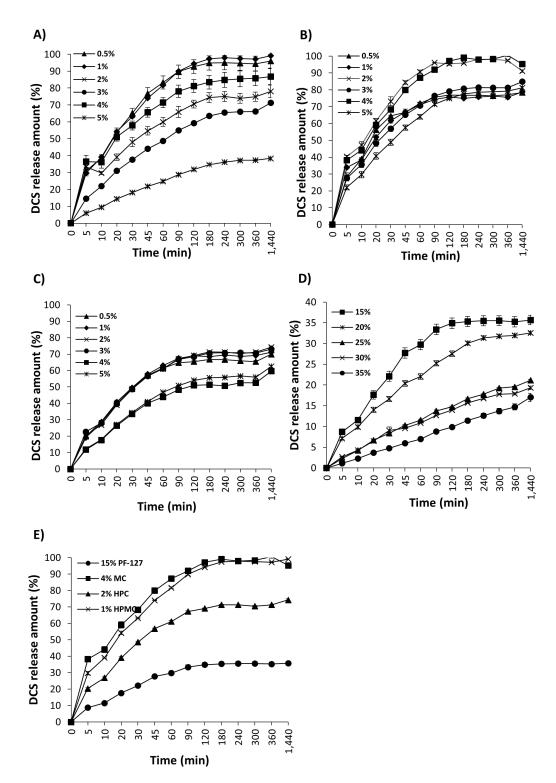
Figure 3. Dissolution of DCS 40 mg/2 mL from polymeric gels. *In vitro* DCS release behavior from (A) HPMC, (B) MC, (C) HPC and (D) PF-127 gel was analyzed with the Distek dissolution apparatus and HPLC. (E) Comparison of *in vitro* DCS release behavior of four polymeric gels (HPMC, MC, HPC and PF-127). The data are expressed as a function of time (min) versus cumulative DCS release amount (%). Data are expressed as mean  $\pm$  standard deviation (n = 3).
