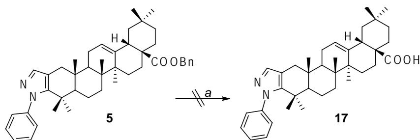
**Scheme 2.** Reagents and conditions: a) H<sub>2</sub>, 10% Pd-C, AcOH/1M HCl, r.t.
