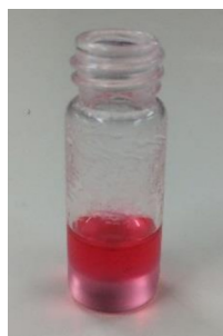
Figure 5. Partition in phase separated solution of poly (lactic-co-glycolic) acid (PLGA)-Suppcire ® AM-methylene chloride. Poly (lactic-co-glycolic) acid (PLGA) and Suppcire AM (200 mg each) were dissolved in 0.3 g 0.02% Oil Red O-methylene chloride, and resultant solution was centrifuged.
